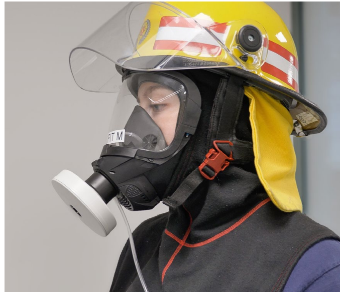
The Draeger FPS7000 is converted to negative pressure mode, using an adaptor, sampling tube, and filter, to enable fit testing.
