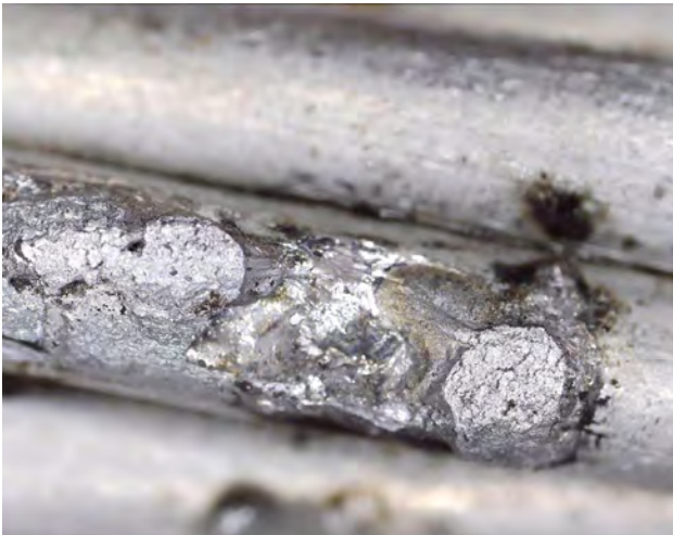
Microscope images of arcing damage on twisted lines.
