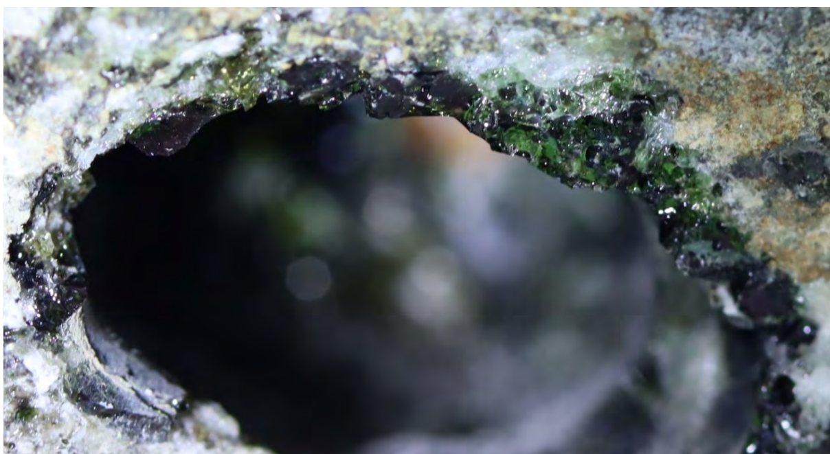
Fig. 70. Cropped IMG 1449JPG – edge of hole has melted like glass.
