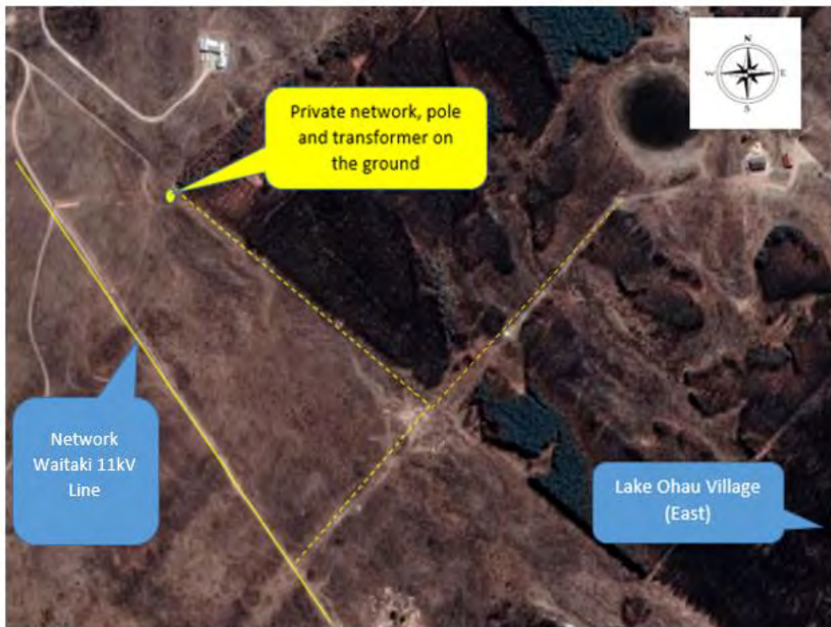
Fig. 4. Image above identifies Network Waitaki 11kV lines (solid yellow line) and the private network (dotted yellow lines). The Network Waitaki infrastructure was positioned along the maintenance track used to access the investigation start point.
