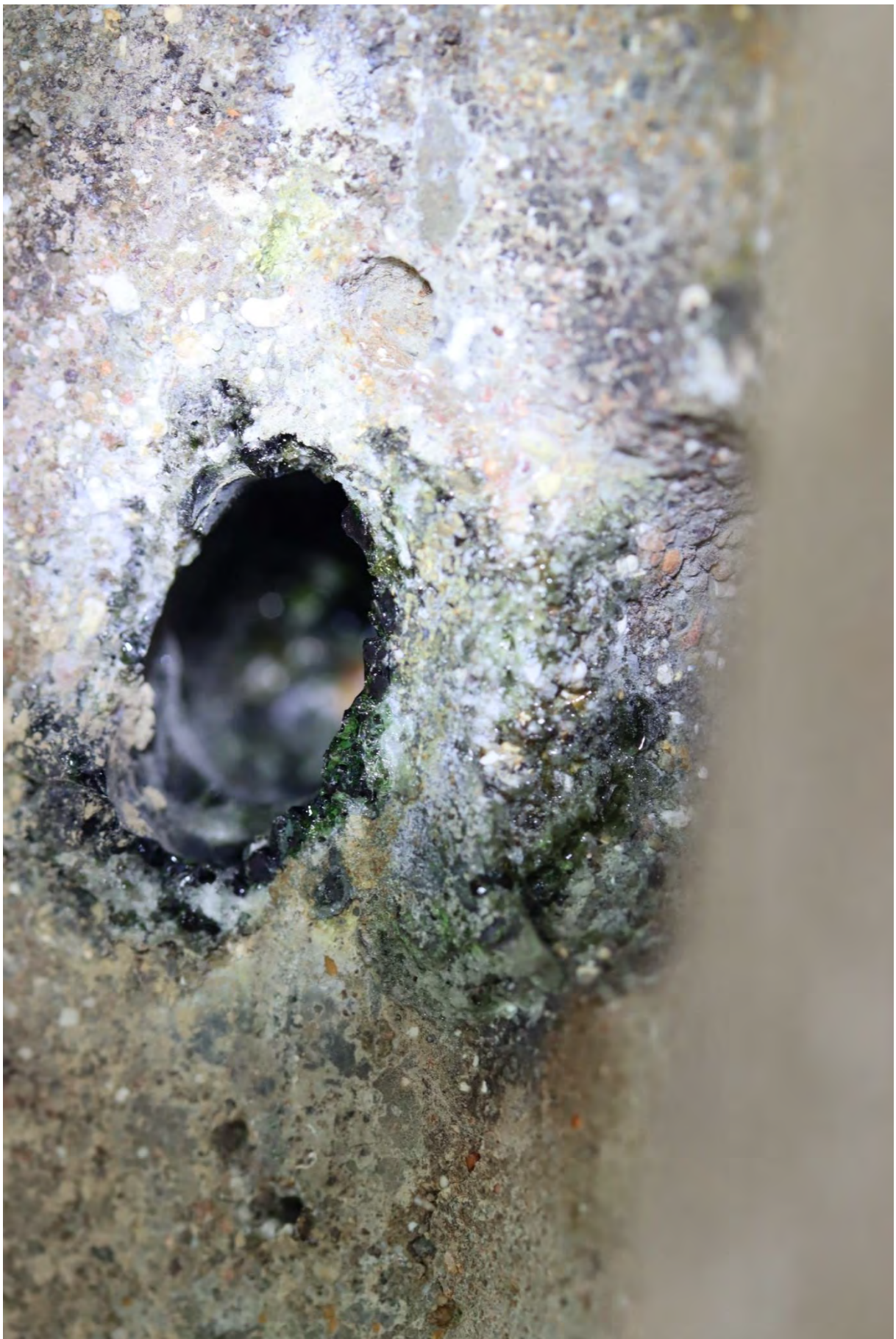
Fig. 71. IMG_1449.JPG edge of hole and surface of pole has been exposed to intense heat.
