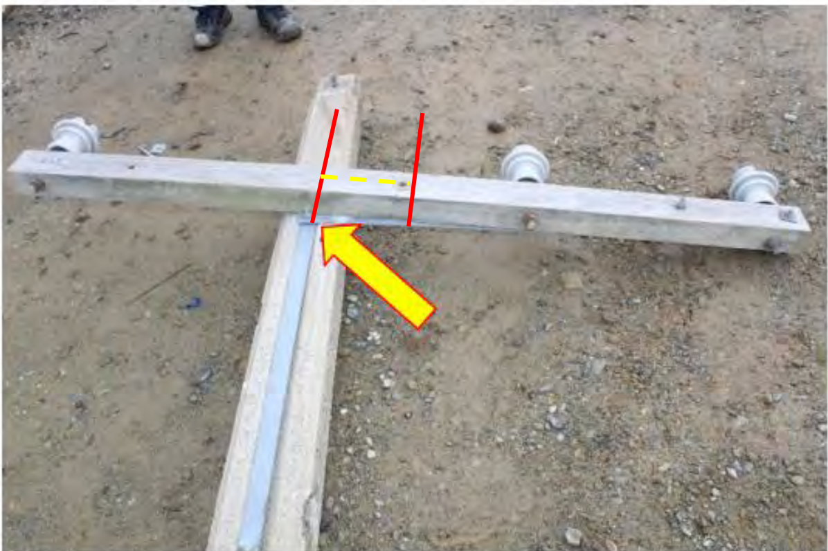
Fig. 59. Above, balancing position of wooden cross-arm after centre bolt vibrated backwards. Note: crossarm has displaced towards the hill side (right of pole) by approximately 250mm off centre.
