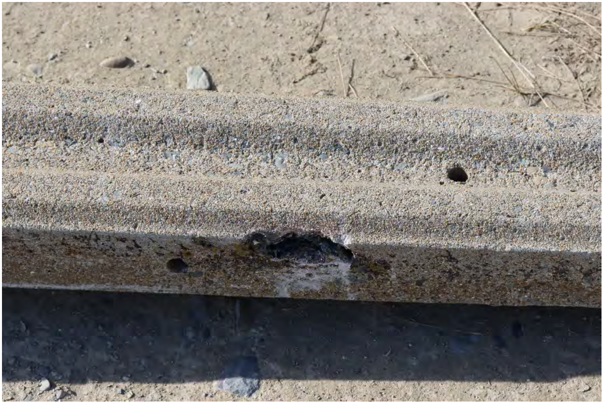
Fig. 78. Old damage on side of pole that lines up with the cross-arm when twisted over. IMG_1415.JPG.
