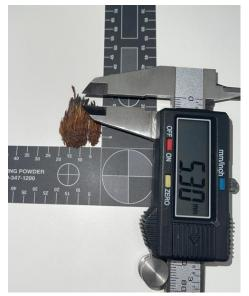
**Fig. 10.** The tips of the vegetation were burnt measuring approximately 5mm. The rest of the vegetation had a scorched discoloured appearance. On checking the surrounding area, I couldn't locate any vegetation that matched.
