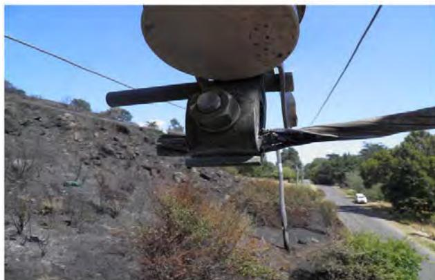
Although time-lines are unknown, the clamp condition must have been less than ideal for quite some time before the overcurrent event on 13 February 2017. I say this because if the clamp had conducted normal load currents (and the overcurrent), equally through all the Aluminium cores of the Flounder overhead conductor then three of the cores would not have arced and severed as shown in the Photograph .
