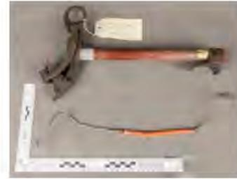
NZ Police photo 17ch0873-0404 showing what they believe to be the red phase fuse carrier and fuse. The fuse looks like a ruptured White phase fuse shown on the pole.
