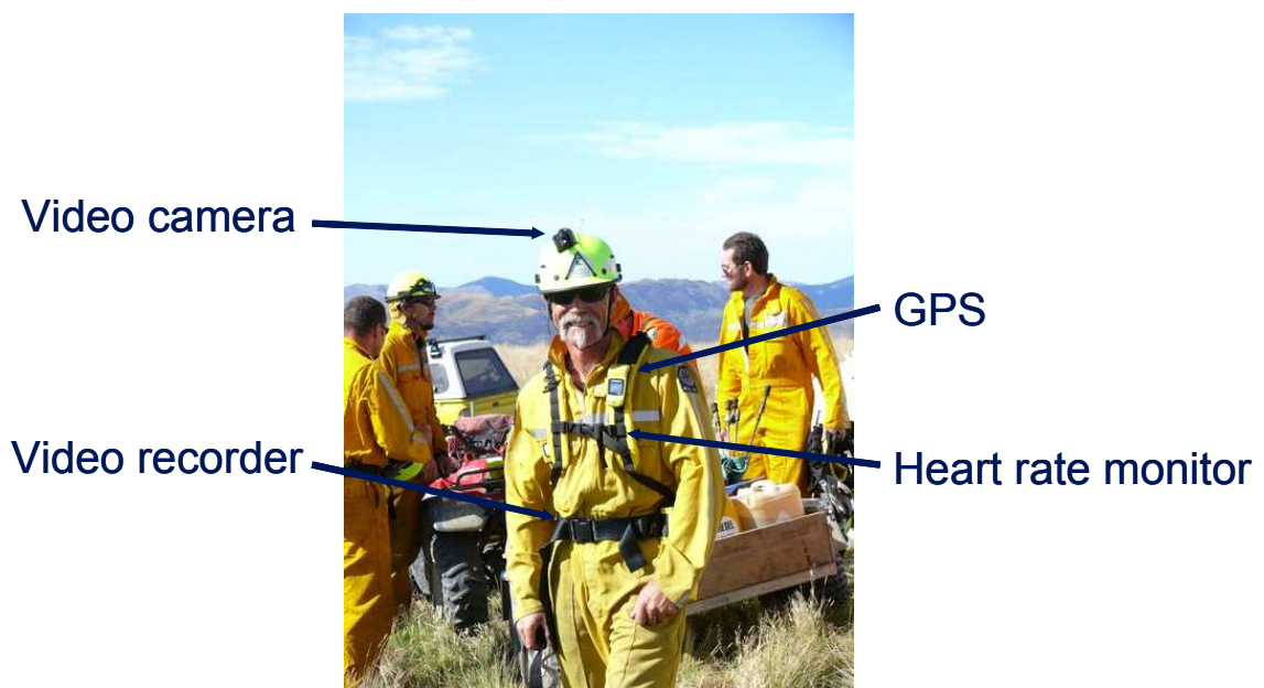
Data collection harness for rural fire fighter
