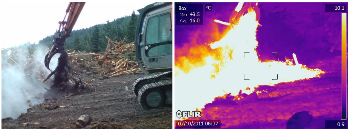
Image 7. Example showing thermal imaging and heat in a slash pile. The DOC FLIR 620 high resolution thermal camera was used to scan a super-skid of concern. Temperatures ranged between 20–60°C, indicating the early stage of organic decomposition (B. Janes, FENZ).
