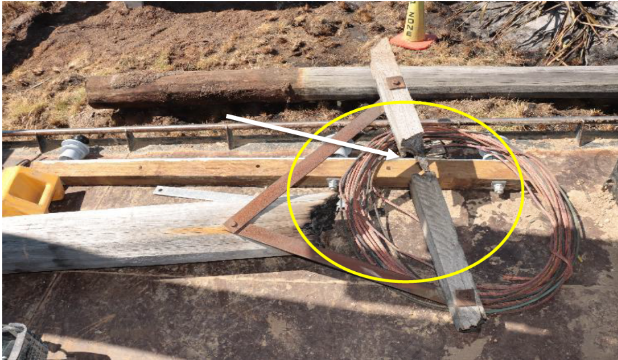
Photo 13: White arrow shows where the fire burnt through the crossarm, yellow circle indicates the burnt away section of the top of the pole.
