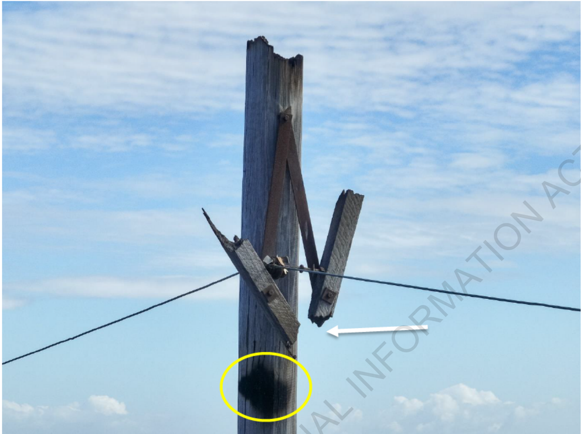
Photo 15: Yellow circle shows where a powerline was striking the power pole after the crossarm broke. White arrow shows burnt away tips of the crossarm.
