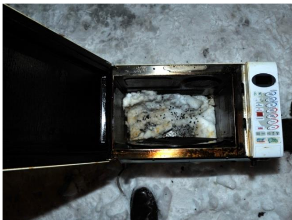
Results of an overheated wheat bag which was inadvertently heated in a microwave oven for 20 minutes
