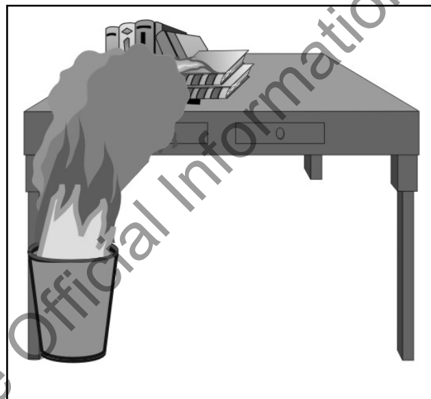
Figure 2.9: Transfer of fire / heat by direct burning or direct flame contact
