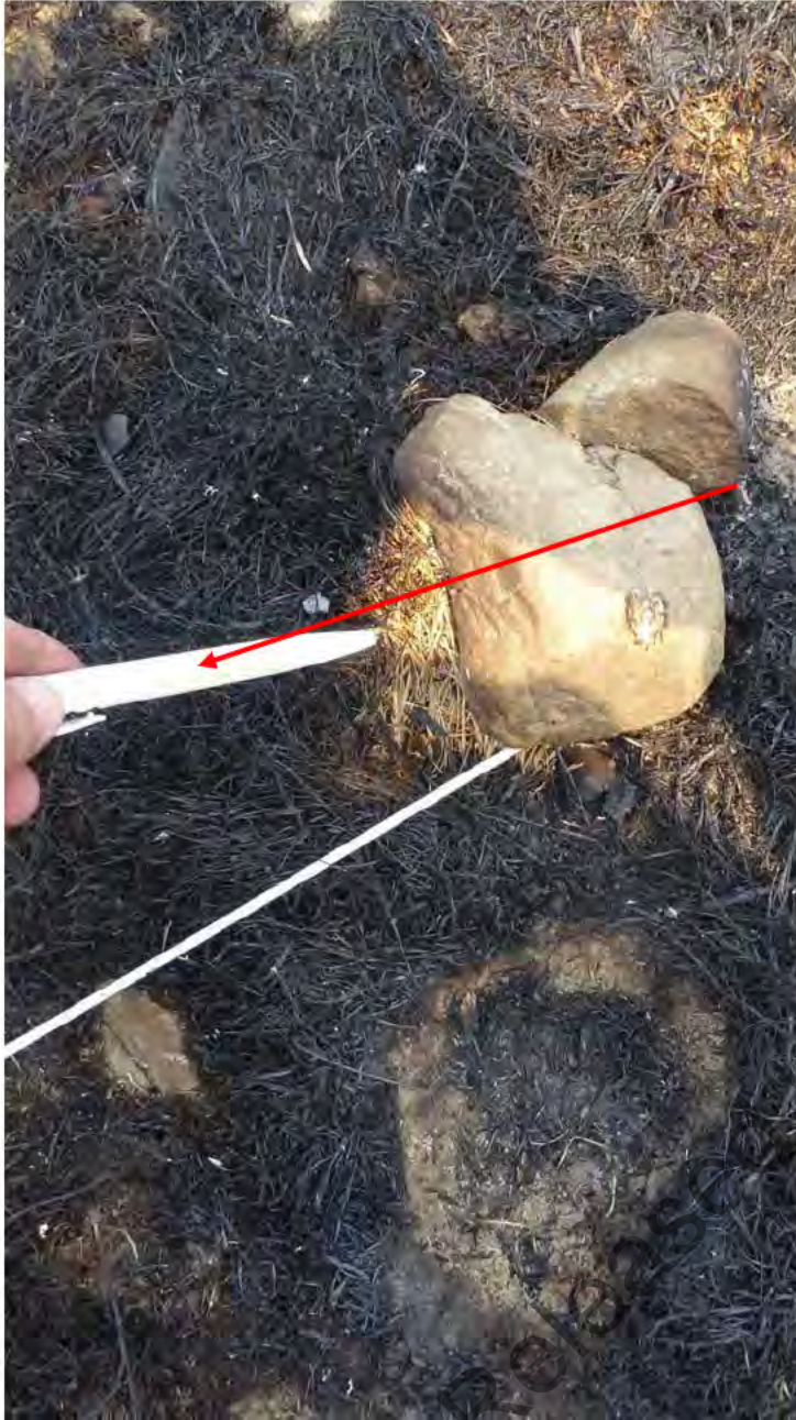
28, Photo 811, 812, 813 – Advancing vector indicators. Protection in lee of rock. Protection under rock with clean burn line on advancing side.
