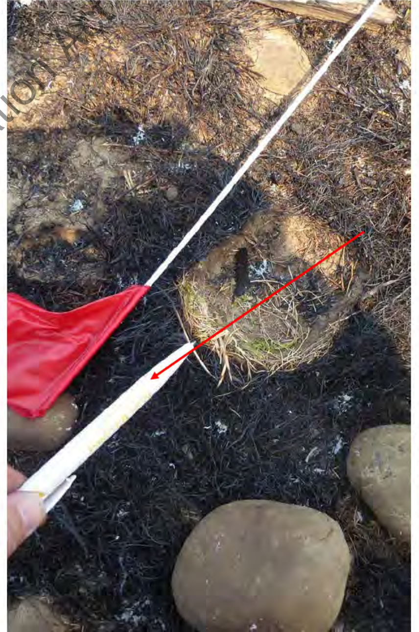
28, Photo 811, 812, 813 – Advancing vector indicators. Protection in lee of rock. Protection under rock with clean burn line on advancing side.
