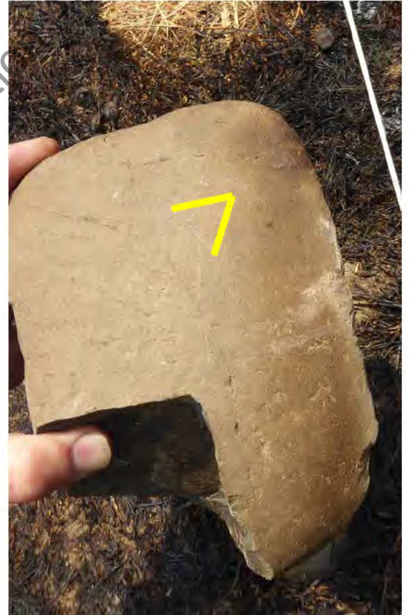
29, Photo 816, 817, 818 – Lateral vector indicators. Protection in lee of rock. Protection under rock with clean burn line on advancing side. Staining on lateral advancing side of rock
