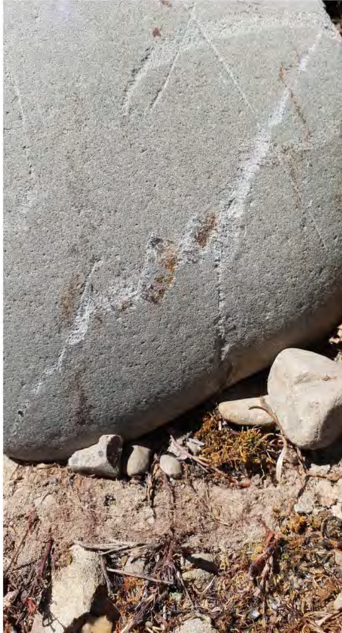
14, Photos 20190213-153053, -150838, -150632. Examples of the amount of metal smeared onto rocks by the discs outside of the origin area.
