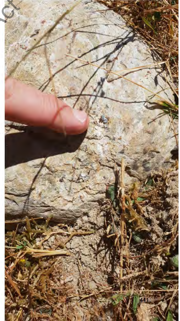
14, Photos 20190213-153053, -150838, -150632. Examples of the amount of metal smeared onto rocks by the discs outside of the origin area.
