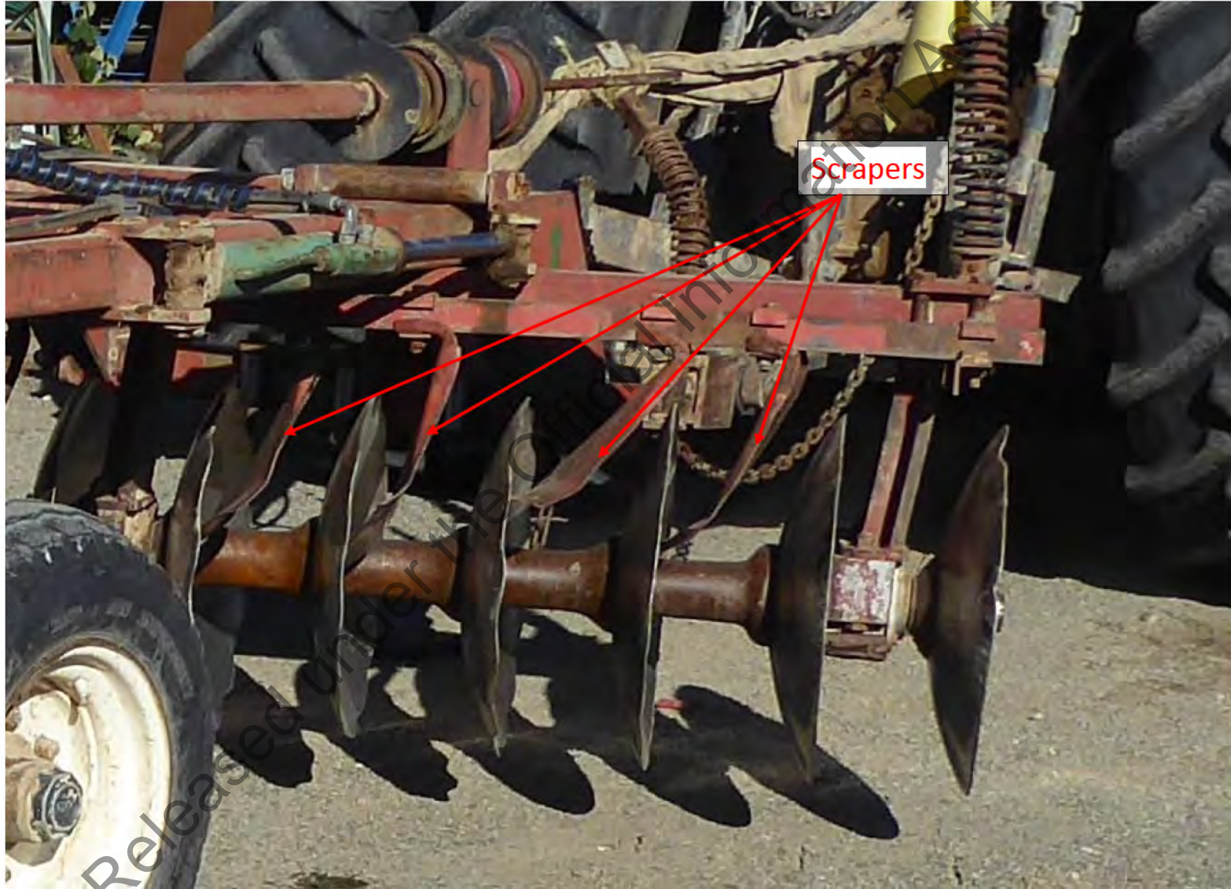
8, Photo 795. Close up of discs and scrapers. (Note scrapers are bent and out of alignment, this shows the wear and tear on scrapers as part of normal operations.)
