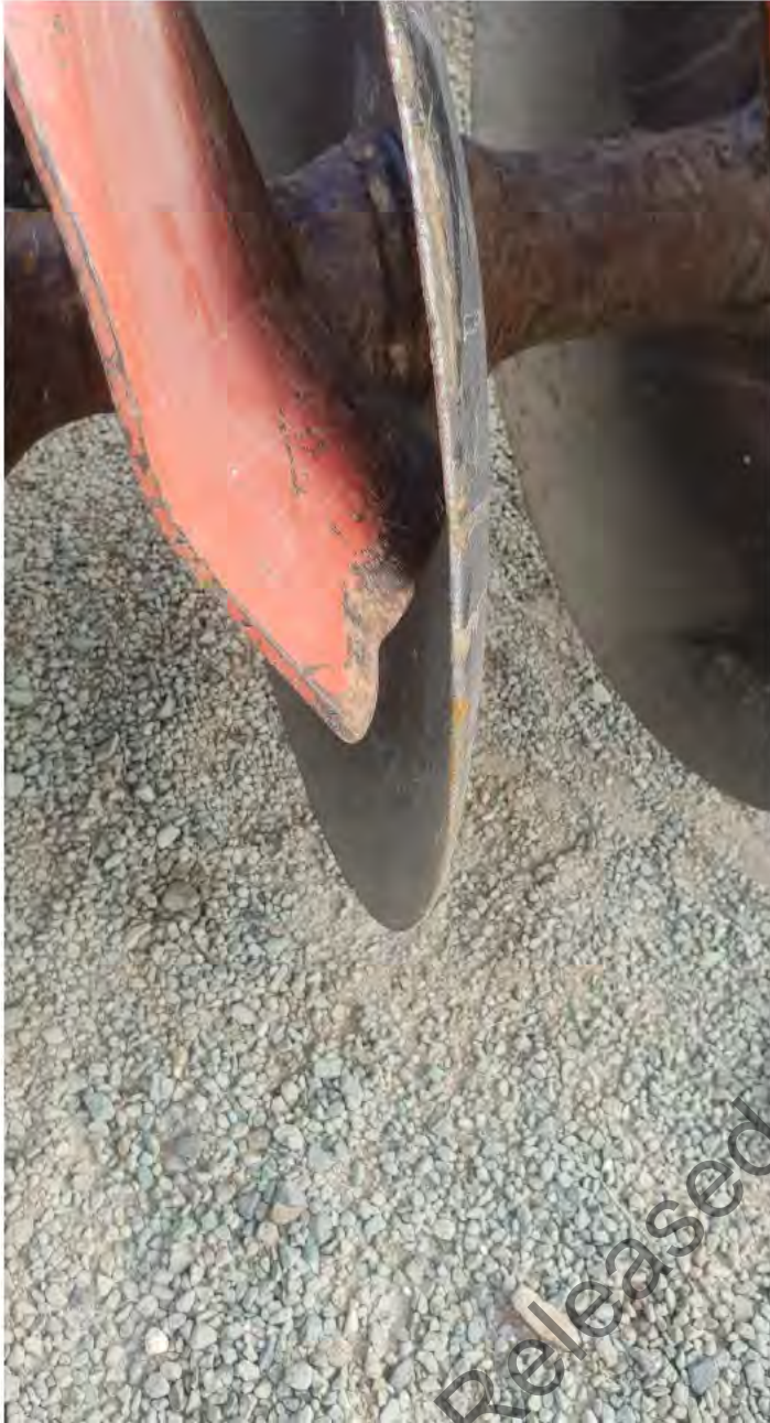
9, Photos 20190214-091241,-091301,-094037. Close up of discs and scrapers. (Note scrapers are at different distances from discs and in some cases very close.)
