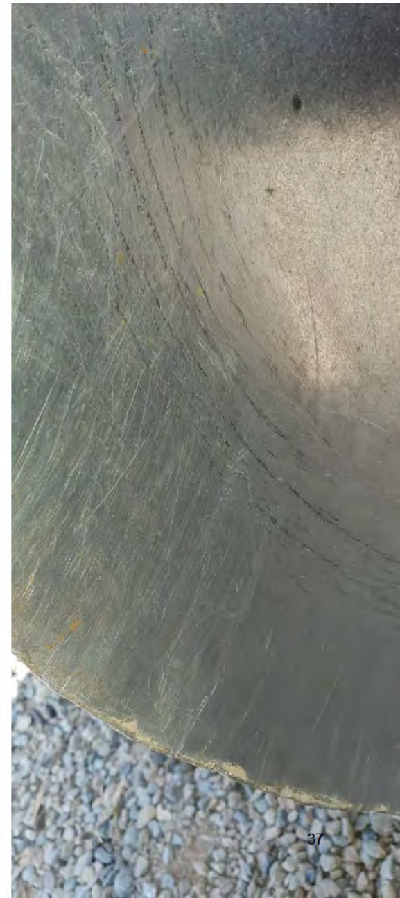
10, Photos 20190214-094156,-094208,-104817,-102140. Close up of fresh abrasion to scraper and corresponding scratches in disc. (3 rd disc and scraper set in from front right gang)
