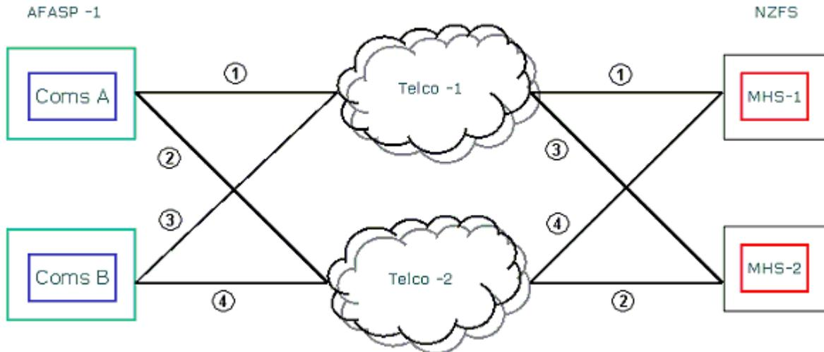
Figure 2 represents all the communication paths required for a single application protocol implementation. Each of the AFASP communication servers and FENZ STSMHS domain servers is connected via two links to the other servers. Each link is an FENZ AFASP API protocol link. With all three protocols running, there are a total of 12 ( $3 * 4$ ) paths between two AFASP systems and two FENZ STSMHS domain servers.
