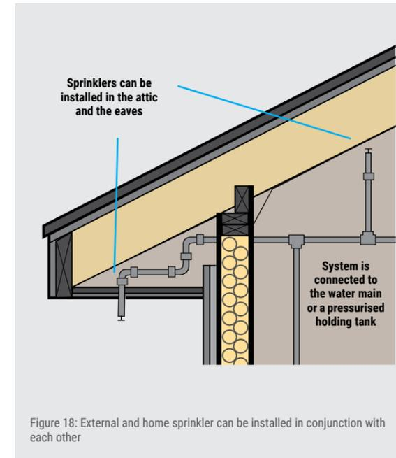
Figure 18: External and home sprinkler can be installed in conjunction with each other
