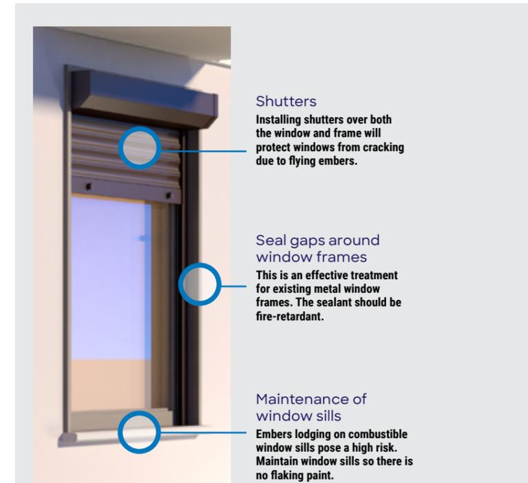
Figure 13: Recommended window protection
