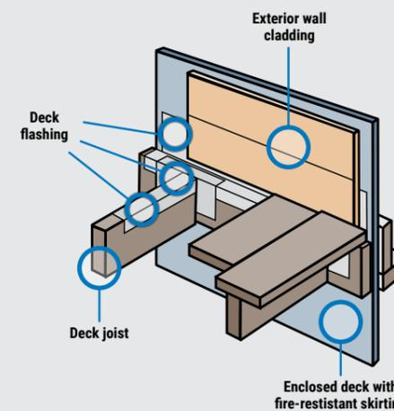
Figure 16: Deck flashing
