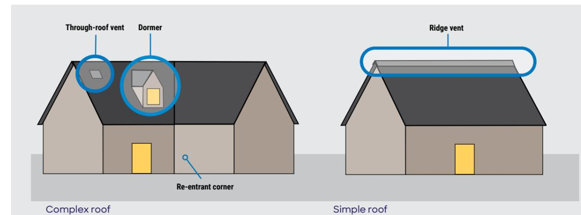
Figure 5: Complex versus Simple roof design
