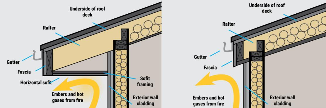
Figure 8: An eave with essentially no overhang versus an enclosed overhang with horizontal soffit
