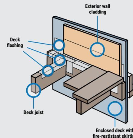
Figure 16: Deck flashing
