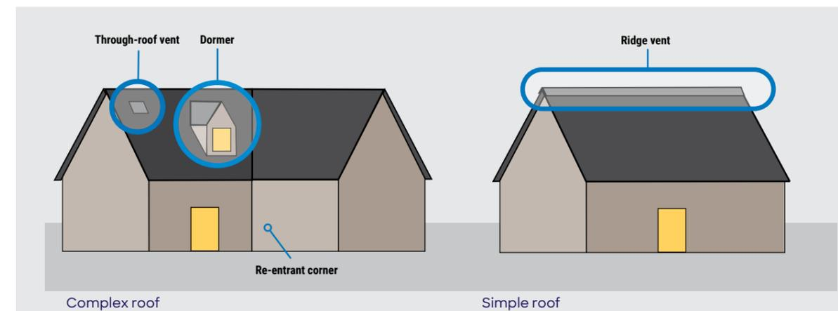
Figure 5: Complex versus Simple roof design
