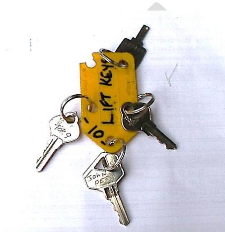
Figure 4: Fire service lift control keys
