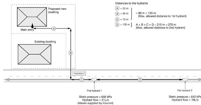
**Figure 2: Firefighting water supply requirements for a non-sprinklered house with access to a reticulated supply**
