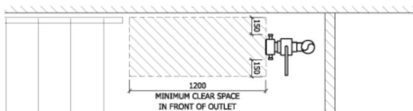
**Figure 14: Car park building hydrant clearance**
