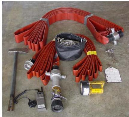
Figure 15: Typical firefighting equipment carried into a multi-storey building
