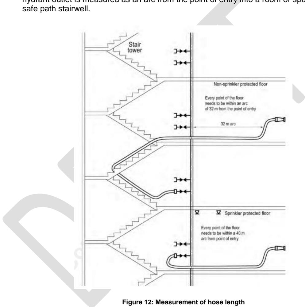
**Figure 12: Measurement of hose length**
