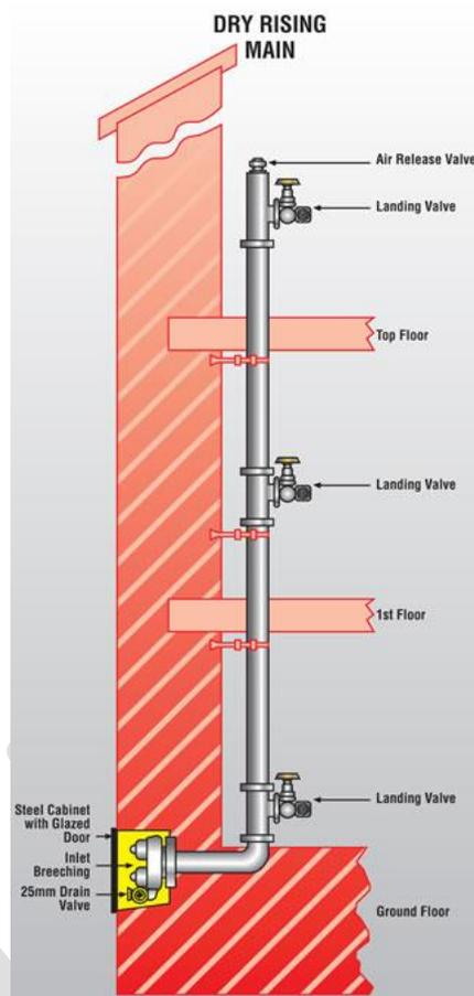
Figure 6: Dry rising main schematic
