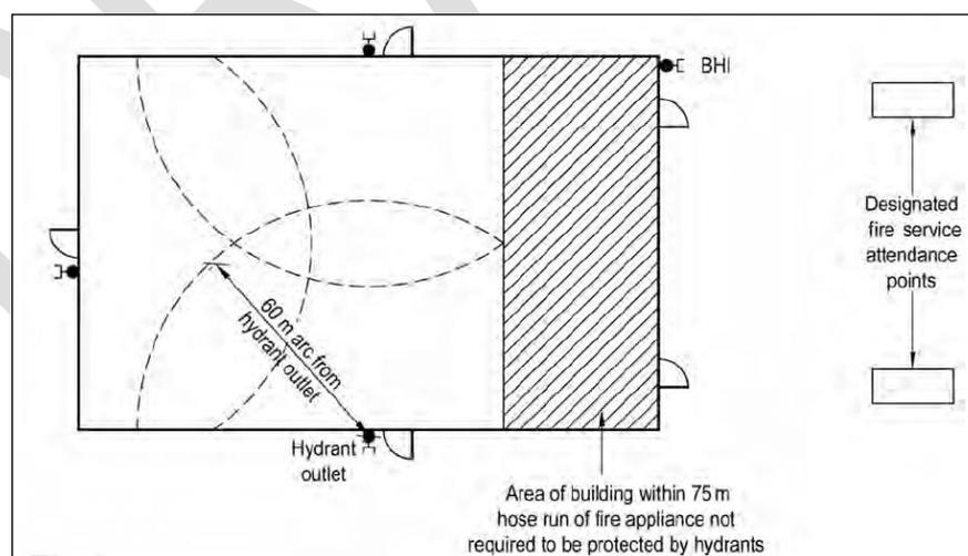
Figure 17: External hydrant outlets and access
