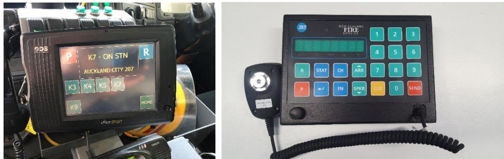
Figure 1 – Shows both a UHF and a VHF LMR terminal
