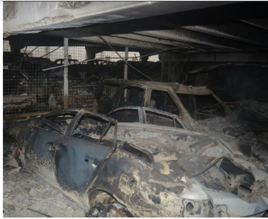
Figure 4 – The aftermath of a fire involving closely stored cars.
