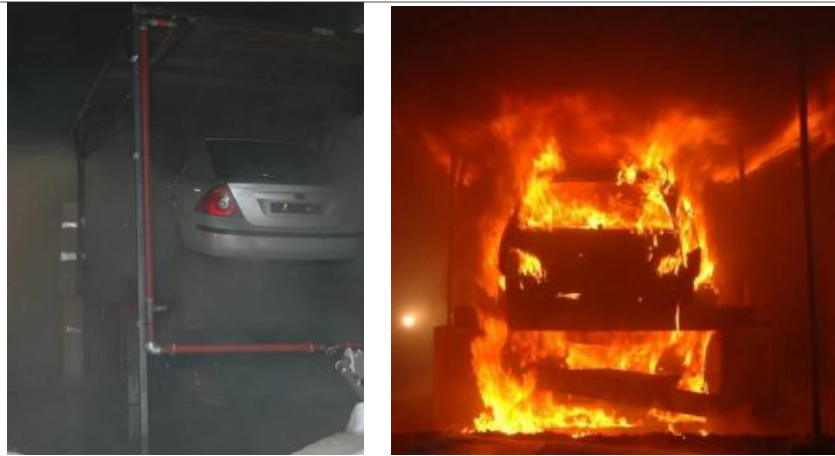
Figure 5 – Conditions in test fires utilising stacked cars
