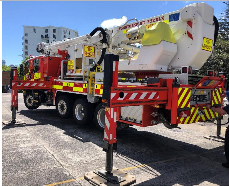
Figure 13 – Highlights the space requirements for jacking stabilisers
