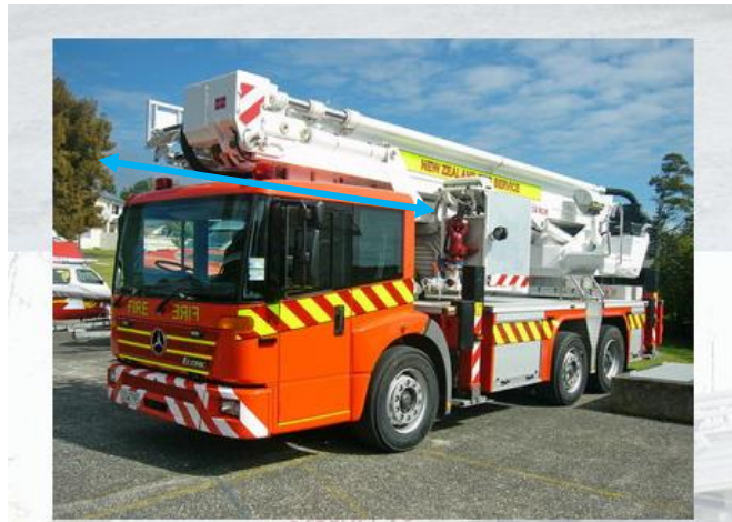
Figure 5 – Showing long front overhang
